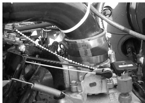
Speed control to throttle attachment (side view)
